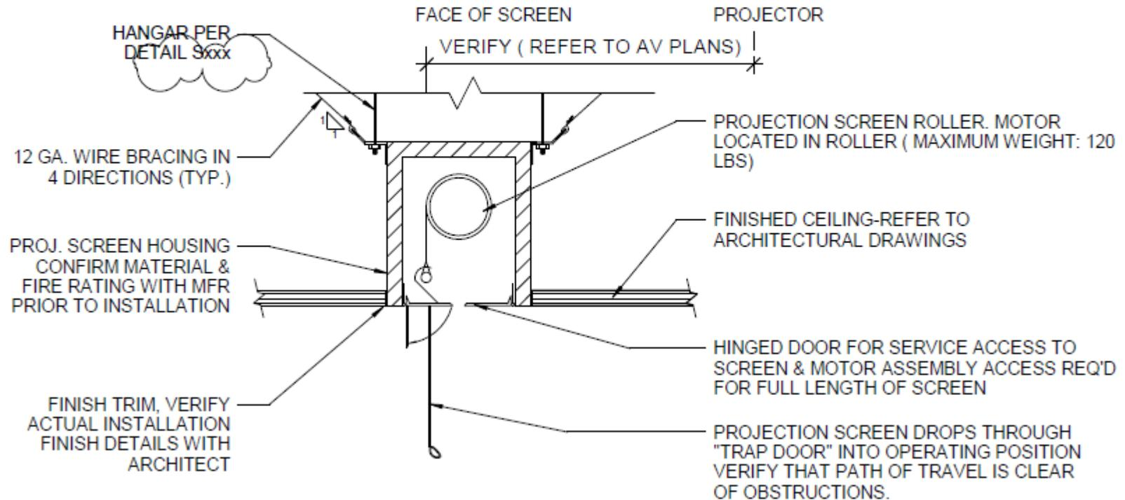
**Ceiling Mounted Projection Screen Detail**
