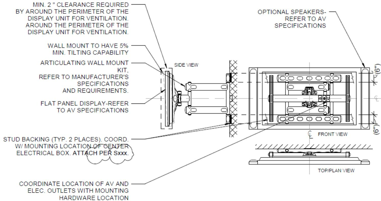
**Wall Mounted Medium - Large Flat Panel Display Detail**
