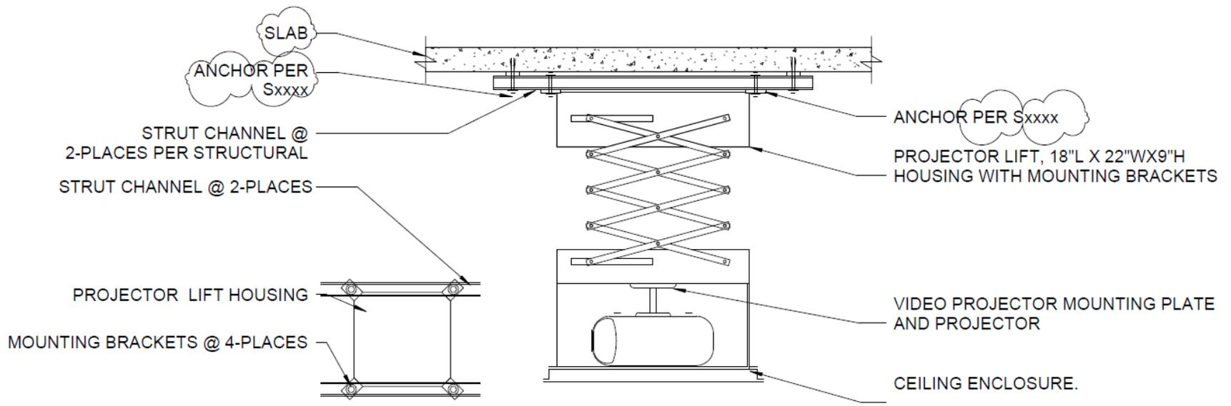
**Ceiling Mounted Projector Lift Detail**
