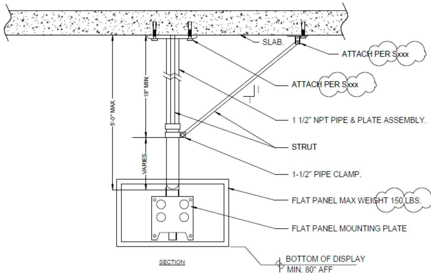
**Ceiling Mounted Flat Panel Display Detail**
